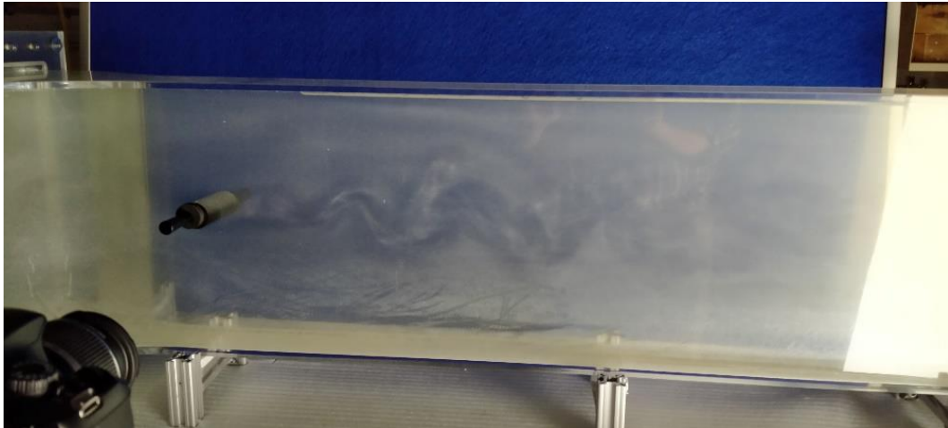
Figure 1: Image of the first test section of the water tunnel with flow visualization particles and a van-Karman street behind a cylinder at flow speed of 15mm/s.
