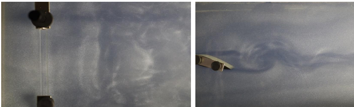
Figure 4: Images of flow visualization of rectangular block situated vertically (left) and Airfoil NACA0024 at 20° angle of attack (right).
