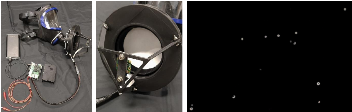
Figure 3: Left: Dräger mask with power bank and single board computer. Center: Inlet with camera mounted on a tripod. Right: Helium-filled soap bubbles (HFSB) captured with the head mounted camera system (enlarged).
