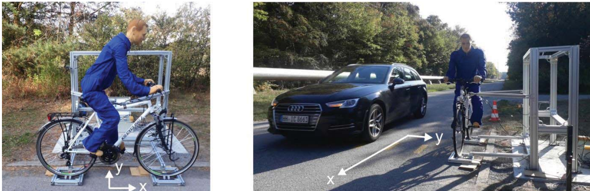
Fig 1: Dummy-bike assembly mounted on rack (left), snapshot of passenger car during overtaking maneuver.
