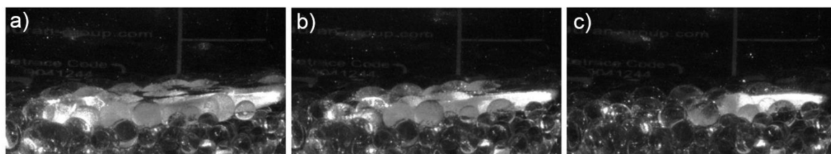
Fig. 2: From left to right, evolution of the ice-like solid structure exposed to non-stability conditions. The structure is illuminated and tracked according to the experimental set-up described in Fig. 1c.
