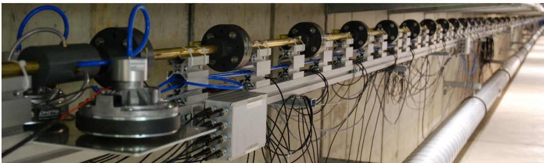
Figure 5: A 48-m-long pipe section (3200 D) with 36 hot wires is connected downstream of the disturbance system
