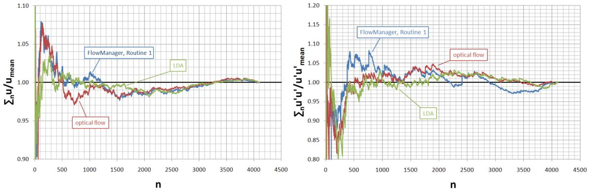
Figure 3: Convergence of the velocity component  $u$  (left) and the fluctuation  $u'u'$  (right) for high turbulence case
