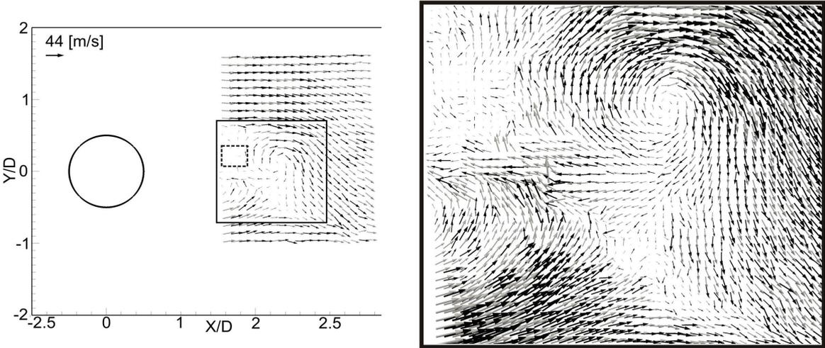
Figure 5: Instantaneous PIV-Measurement, processed with cross correlation.
