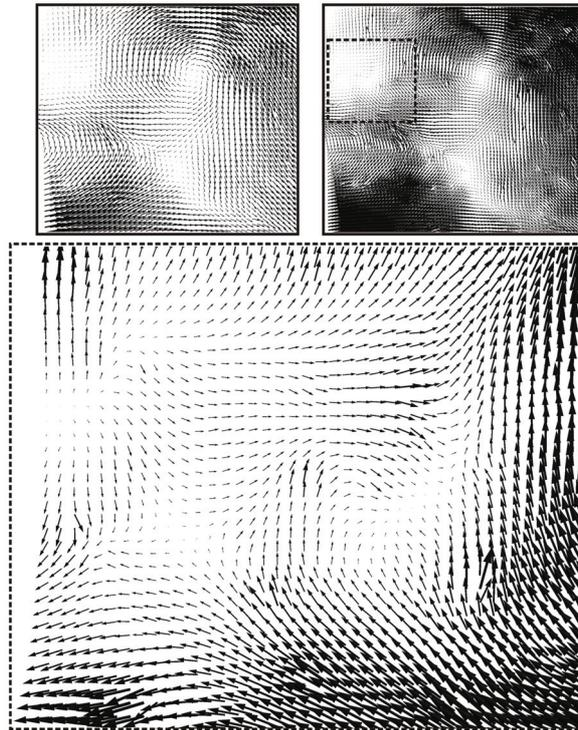
Figure 6: Instantaneous PIV measurement, processed with Optical Flow
