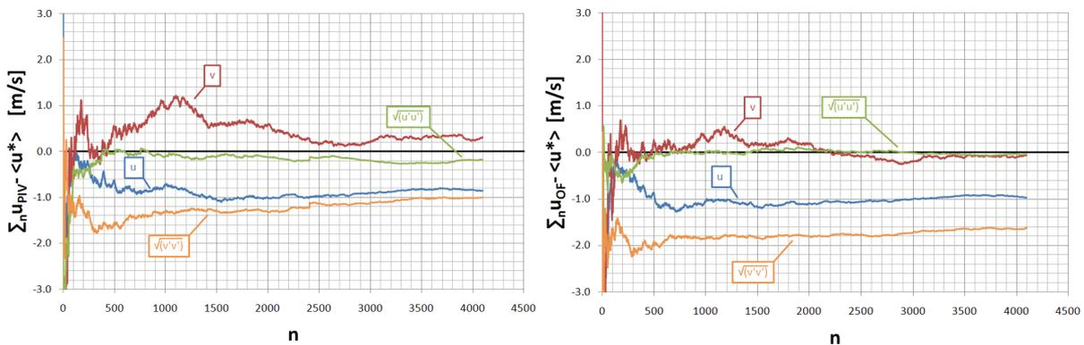
Figure 4: Convergence of the difference of the velocity components and the fluctuations to the converged LDA results for Cross Correlation with FlowManager (left) and Optical Flow (right) at the high turbulence case.
