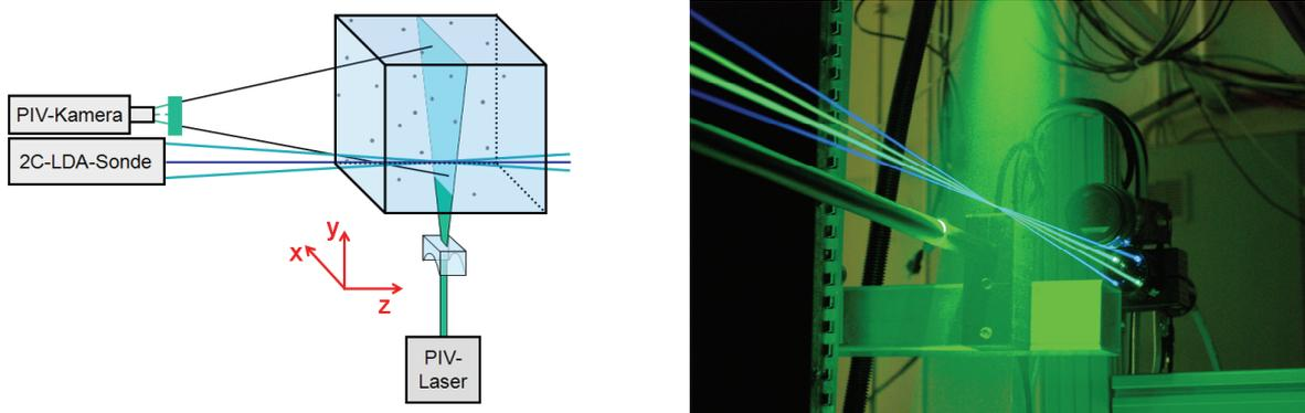
Figure 1: Principle setup of simultaneous PIV/LDA-measurements.
