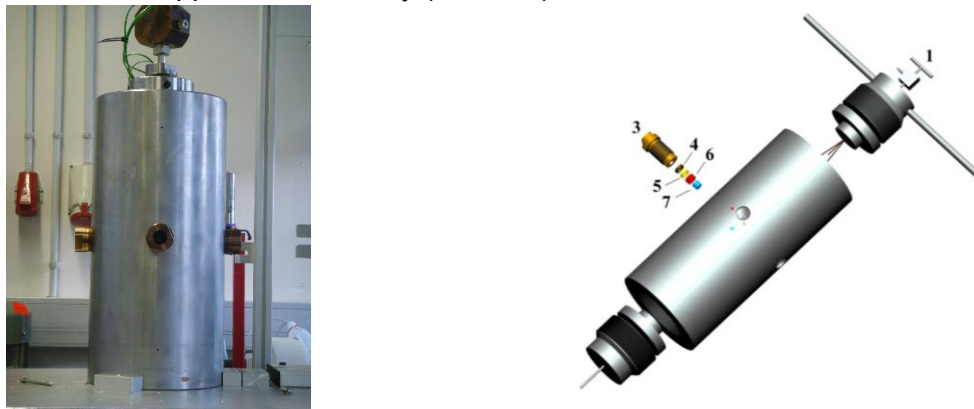
Fig. 2 Photograph (left) and technical drawing (right) of high pressure vessel with optical windows
