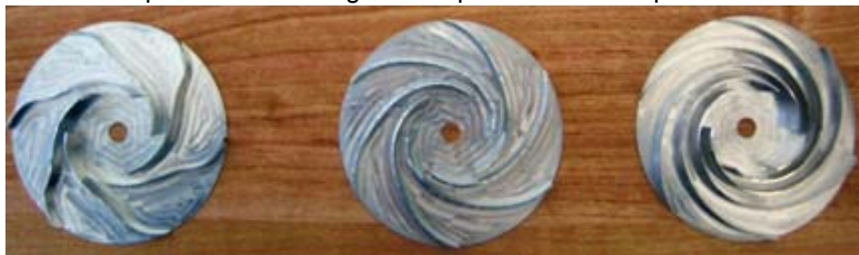
Figure 5: Prototypes of impellers with wrap angles \theta=120^\circ , 150^\circ and 228^\circ
