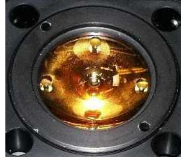
Fig. 3b: The frontside view of the injection molded polycarbonate lens, with four integrated collimating lenses on the surface and a secondary centric mirror inside (Au-coated for 980nm).
