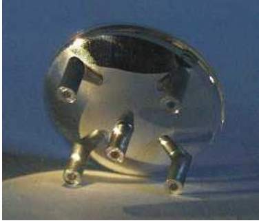
Fig. 3a: The backside view of the injection molded monolithic polycarbonate lens, with five tubes for guiding the optical fibers (Al-coated for 532 nm)
