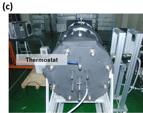
Fig. 1: Deep sea simulator together with the PIV system (a)-(c). High pressure vessel dimensions in cm (b). System diagram of the high pressure vessel and the cooling tank (d).
