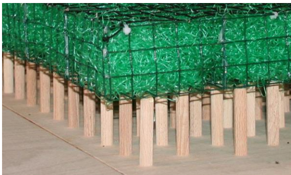
Figure 1: Wind-tunnel forest model.
