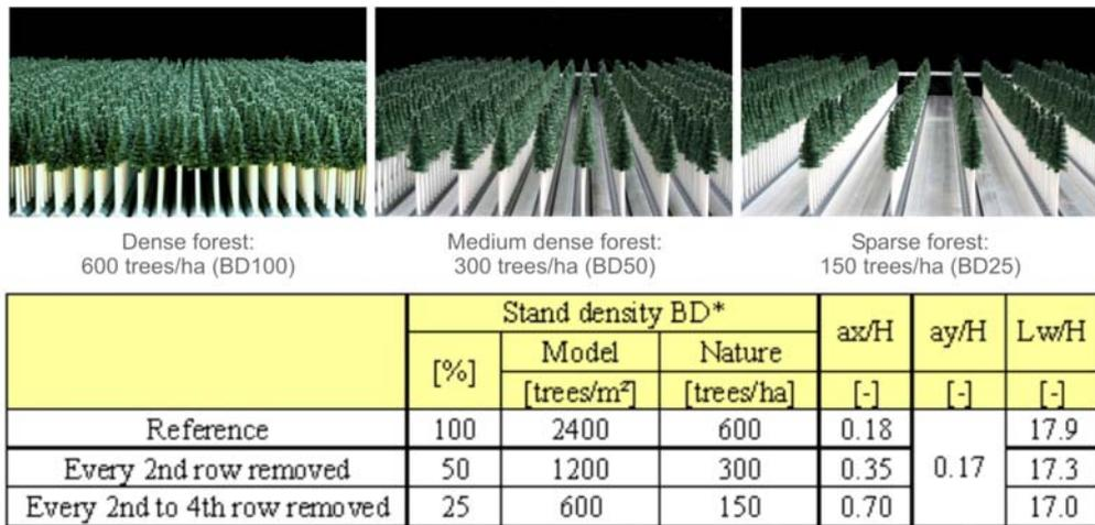
Figure 1: Homogenous forest stands: outline of tests;  $ax$  = spacing between the trees in stream-wise direction,  $ay$  = spacing between the trees in lateral direction (perpendicular to the approach flow),  $Lw$  = length of the forest = distance between first and last tree row,  $H$  = mean stand height = 23 m, \*stand density based on the ground area of the reference configuration
