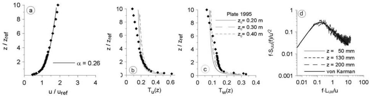
Figure 3: Simulated atmospheric boundary layer: a) time-averaged horizontal velocity  $u(z)$  ( $z_{\text{ref}} = 0.05 \text{ m}$ ,  $u_{\text{ref}} = 4.34 \text{ m/s}$ ), b) turbulence intensity in main flow direction  $T_u(z)$ , c) Turbulence intensity in vertical direction  $T_w(z)$ , d) Normalized spectral density functions  $f \cdot S_{uu}(f)/u^2$
