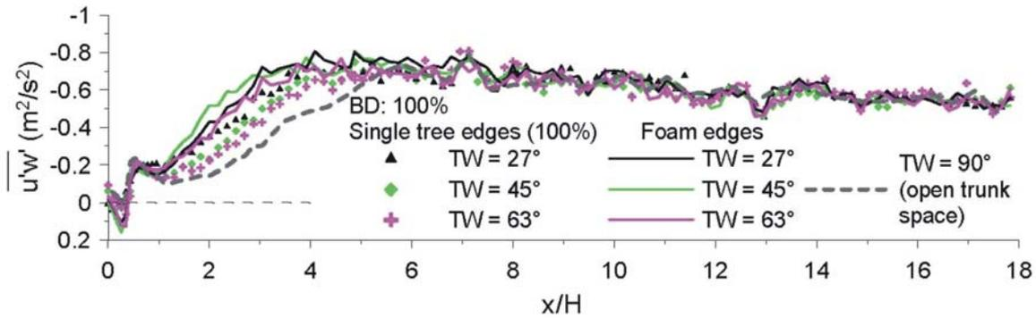
Fig. 5 Dependency of time-averaged turbulent momentum flux  $\overline{u'w'}$  close to the canopy top ( $z/H = 1.13$ ) above a dense stand (BD100) on different windward forest edges
