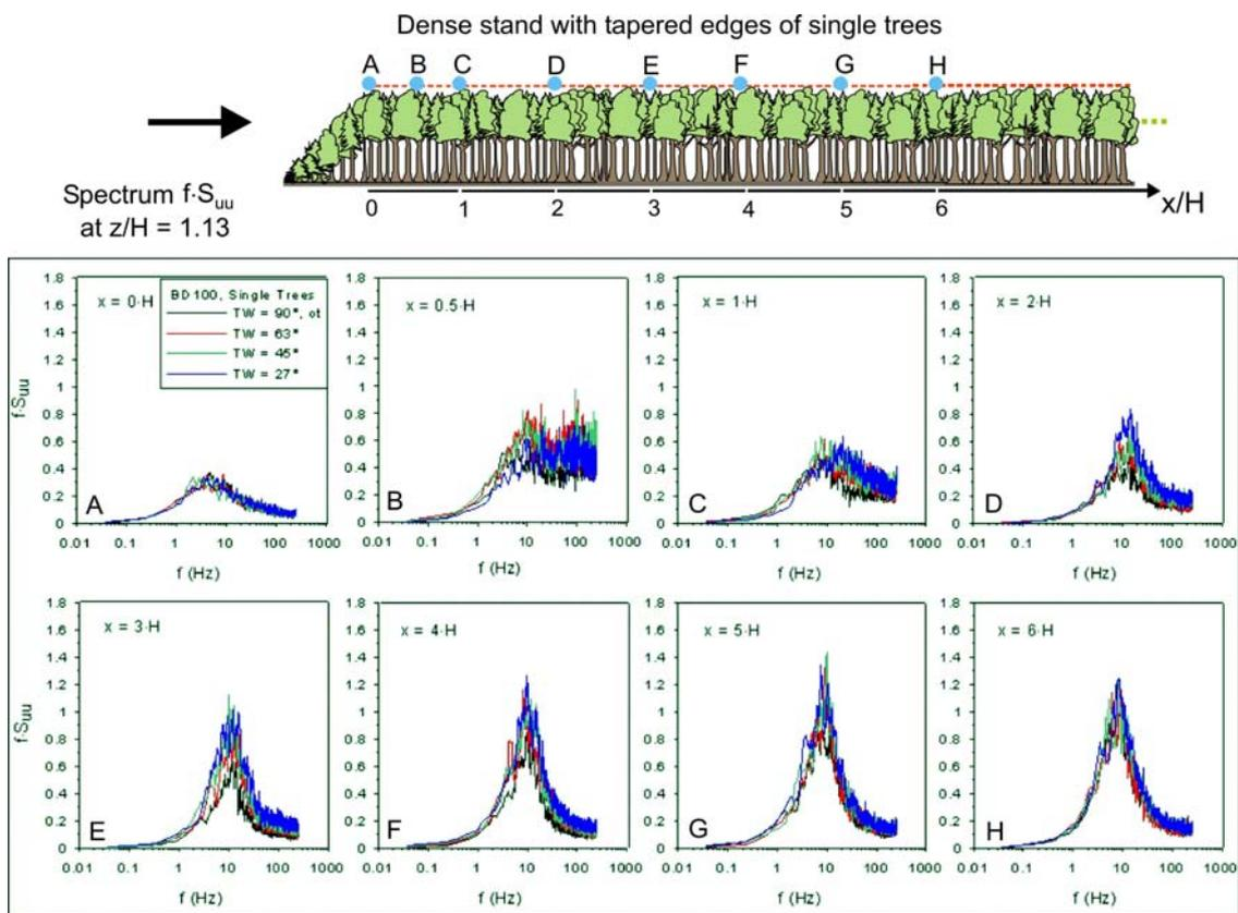
Fig. 7: Spectrum of horizontal streamwise wind fluctuations close to the canopy of a dense forest with tapered edges, tree density BD100, taper angle  $27^\circ$ ,  $45^\circ$ ,  $63^\circ$ ,  $90^\circ$
