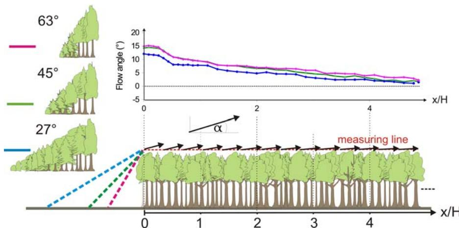
Fig. 4: Flow angle of the time-mean outflow through the canopy, measured at  $z/H=1.13$ ; tapered edges consisting of single trees, tree density BD100, taper angle  $27^\circ$ ,  $45^\circ$ ,  $63^\circ$
