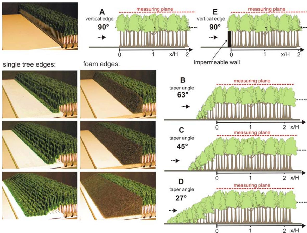
Figure 2: Forest models with different edge structures: A) forest edge with open trunk space; B), C), D) single tree edges with taper angles  $TW=63^\circ, 45^\circ, 27^\circ$ , E) figure of dense forest with impermeable wall
